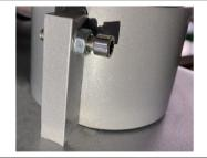
After ten thousands of swing-away and press, maybe you need to adjust the position screw on the back column to make sure the upper heating platen and lower platen is always paralleled. (For Air Pro One and X)
